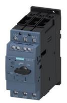
Circuit breaker size S2 for motor protection, CLASS 10 A-release 32...40 A N-release 585 A screw terminal Standard switching capacity with transverse auxiliary switches 1 NO+1 NC
