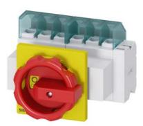
SENTRON, Switch disconnector 3LD, emergency switching-off switch, 6-pole, Iu: 25 A, operating power / at AC-23 A 400 V: 9.5 kW, front-mounted, 1 NC, 1 NO, rotary operating mechanism, Red / yellow, 4-hole mounting of the handle
