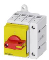
Load disconnector 3LD3, lu 63 A Main switch 3-pole + N Rated operating capacity at AC-23 A at 400V 22.0 kW Installation in distribution boards, Basic switch with selector knob red / yellow
