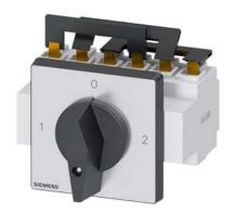
SENTRON, Switch disconnector 3LD, change-over switch, 3-pole, lu: 63 A, Operating power / at AC-23 A at 400 V: 22 kW, front-mounted, knob-operated mechanism, black, 4-hole mounting of the handle
