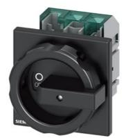
SENTRON, Molded case switch 3LD5 UL, Main switch, 3-pole, certified according to UL489 UL60947-4-1 and IEC60947-3, UL: 30A, SCCR 50kA at 480VAC, Operating power at 480VAC 3-phase: 20hp, IEC: 32A, Operating power at AC-23A at 400V: 15kW, front-mounted, rotary operating mechanism, black, 4-hole mounting of the handle, incl. terminal covers for the infeed side
