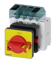
Load disconnector 3LD3, lu 63 A Main switch 3-pole + N Rated operating capacity at AC-23 A at 400V 22.0 kW Front plate mounting Basic switch with Central hole mounting 22.5mm Toggle drive red / yellow 48x48 mm with auxiliary switch 1OE + 1S
