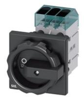
Load disconnector 3LD3, lu 16 A Main switch 3-pole Rated operating capacity at AC-23 A at 400V 7.5kW Front plate mounting Basic switch with Central hole mounting 22.5mm Rotating drive black 66 x 66 mm
