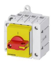
Load disconnector 3LD3, Iu 40 A Main switch 3-pole + N Rated operating capacity at AC-23 A at 400 V 18.5 kW Installation in distribution boards, Basic switch with selector knob red / yellow with auxiliary switch 1OE + 1S
