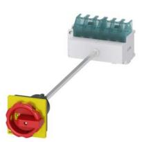
SENTRON, Switch disconnector 3LD, emergency switching-off switch, 6pole, Iu: 25 A, operating power / at AC-23 A 400 V: 9.5 kW, floor mounting with door coupling, 1 NC, 1 NO, rotary operating mechanism, Red / yellow, 4-hole mounting of the handle
