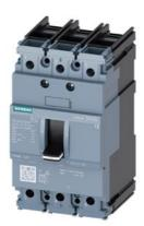
circuit breaker 3VA5 UL frame 125 breaking capacity class H 65kA @ 480 V 3-pole, line protection TM210, FTFM, ln=25A overload protection Ir=25A fixed short-circuit protection li=12 x In UL489 SB (naval), 50 deg. cel. cable connection on both sides
