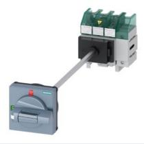
SENTRON, Molded case switch 3LD5 UL, Main switch, 4-pole, certified according to UL489 UL60947-4-1 and IEC60947-3, UL: 30A, SCCR 50kA at 480VAC, Operating power at 480VAC 3-phase: 20hp, IEC: 32A, Operating power at AC-23A at 400V: 15kW, floor mounting with door coupling rotary operating mechanism, defeatable, Standard, 4-hole mounting of the handle, without tolerance compensation, incl. terminal covers for the infeed side
