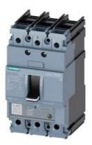
circuit breaker 3VA5 UL frame 125 breaking capacity class M 35kA @ 480 V 3-pole, line protection TM230, FTAM, In=20A overload protection Ir=20A fixed short-circuit protection Ii=7.5...15 x In UL489 SB (naval), 50 deg. cel. cable connection on both sides
