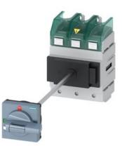
SENTRON, Molded case switch 3LD5 UL, Main switch, 3-pole, certified according to UL489 UL60947-4-1 and IEC60947-3, UL: 100A, SCCR 65kA at 480VAC, Operating power at 480VAC 3-phase: 60hp, IEC: 100A, Operating power at AC-23A at 400V: 45kW, floor mounting with door coupling rotary operating mechanism, defeatable, Standard, 4-hole mounting of the handle, without tolerance compensation, incl. terminal covers for the infeed side
