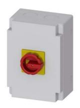
SENTRON, Switch disconnector 3LD, emergency switching-off switch, 3-pole, Iu: 125 A, operating power / at AC-23 A 400 V: 45 kW, Molded plastic encapsulation for inch cable gland, rotary operating mechanism, red/yellow
