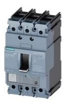
circuit breaker 3VA5 UL frame 125 3-pole, starter protection TM120M, AM, In=10A without overload protection short-circuit protection li=5...12 x In cable connection on both sides
