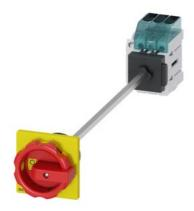
Load disconnector 3LD3, lu 32 A Main switch 3-pole Rated operating capacity for AC-23 A at 400V 11.5kW floor mounting Basic switch with door coupling Central hole mounting 22.5mm Rotary actuator red / yellow 66 x 66 mm with auxiliary switch 10E + 1S
