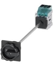
Load disconnector 3LD3, lu 63 A Main switch 3-pole Rated operating capacity at AC-23 A at 400V 22.0 kW floor mounting Basic switch with door coupling Central hole mounting 22.5mm Rotating drive black 66 x 66 mm with auxiliary switch 10E + 1S
