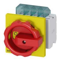
SENTRON, Switch disconnector 3LD, emergency switching-off switch, 4-pole, Iu: 16 A, operating power / at AC-23 A 400 V: 7.5 kW, front-mounted, 1 NC, 1 NO, rotary operating mechanism, Red / yellow, 4-hole mounting of the handle
