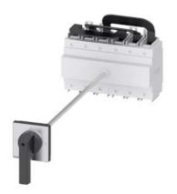
SENTRON, Switch disconnector 3LD, change-over switch, 3-pole, lu = 250 A, Operating power / at AC-23 A at 400 V: 132 kW, floor mounting with door coupling, knob-operated mechanism, black, 4-hole mounting of the handle
