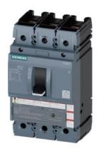
circuit breaker 3VA5 UL frame 250 breaking capacity class C 100kA @ 480 V 3-pole, line protection TM230, FTAM, In=110A overload protection Ir=110A fixed short-circuit protection li=5...10 x In UL489 SB (naval), 50 deg. cel. nut keeper kit on both sides
