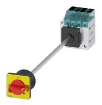
Load disconnector 3LD3, lu 16 A Main switch 3-pole + N Rated operating capacity at AC-23 A at 400V 7.5kW floor mounting Basic switch with door coupling Central hole mounting 22.5mm Toggle drive red / yellow 48x48 mm with auxiliary switch 10E + 1S
