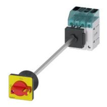
Load disconnector 3LD3, lu 16 A Main switch 3-pole + N Rated operating capacity at AC-23 A at 400V 7.5kW floor mounting Basic switch with door coupling Central hole mounting 22.5mm Toggle drive red / yellow 48x48 mm
