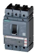
circuit breaker 3VA5 UL frame 250 breaking capacity class H 65kA @ 480 V 3-pole, line protection TM210, FTFM, In=225A overload protection Ir=225A fixed short-circuit protection li=10 x In nut keeper kit on both sides
