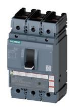
circuit breaker 3VA5 UL frame 250 breaking capacity class C 100kA @ 480 V 3-pole, line protection TM230, FTAM, In=100A overload protection Ir=100A fixed short-circuit protection Ii=5...10 x In UL489 SB (naval), 50 deg. cel. nut keeper kit on both sides
