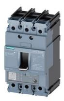
circuit breaker 3VA5 UL frame 125 3-pole, starter protection TM120M, AM, In=3A without overload protection short-circuit protection li=3...7 x In cable connection on both sides
