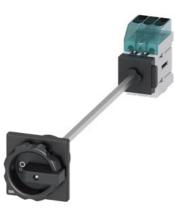
Load disconnector 3LD3, lu 40 A Main switch 3-pole Rated operating capacity at AC-23 A at 400 V 18.5 kW floor mounting Basic switch with door coupling Central hole mounting 22.5mm Rotating drive black 66 x 66 mm
