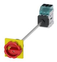
Load disconnector 3LD3, lu 32 A Main switch 3-pole Rated operating capacity for AC-23 A at 400V 11.5kW floor mounting Basic switch with door coupling Central hole mounting 22.5mm Rotary actuator red / yellow 66 x 66 mm
