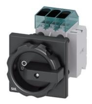
Load disconnector 3LD3, lu 16 A Main switch 3-pole Rated operating capacity at AC-23 A at 400V 7.5kW Front plate mounting Basic switch with Central hole mounting 22.5mm Rotating drive black 66 x 66 mm with auxiliary switch 1OE + 1S
