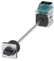
Load disconnector 3LD3, lu 63 A Main switch 3-pole Rated operating capacity at AC-23 A at 400V 22.0 kW floor mounting Basic switch with door coupling Central hole mounting 22.5mm Toggle drive black 48x48 mm with auxiliary switch 1OE + 1S
