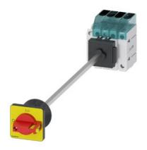
Load disconnector 3LD3, lu 63 A Main switch 3-pole + N Rated operating capacity at AC-23 A at 400V 22.0 kW floor mounting Basic switch with door coupling Central hole mounting 22.5mm Toggle drive red / yellow 48x48 mm with auxiliary switch 1OE + 1S
