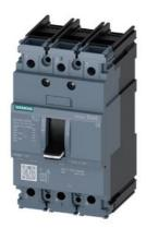
circuit breaker 3VA5 UL frame 125 breaking capacity class S 25kA @ 480 V 3-pole, line protection TM210, FTFM, In=20A overload protection Ir=20A fixed short-circuit protection Ii=15 x In UL489 SB (naval), 50 deg. cel. nut keeper kit on both sides
