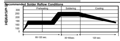
• Recommended reflow methods : IR, vapor phase oven, hot air oven. · Devices are not designed to be wave soldered to the bottom side of the board.
