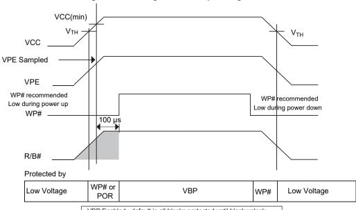
VBP Enabled - default is all blocks protected until block unlock commands define an unlocked range
