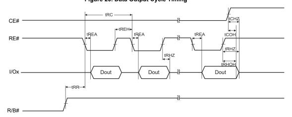
Figure 20. Data Output Cycle Timing<sup>[47, 48, 49]</sup>
