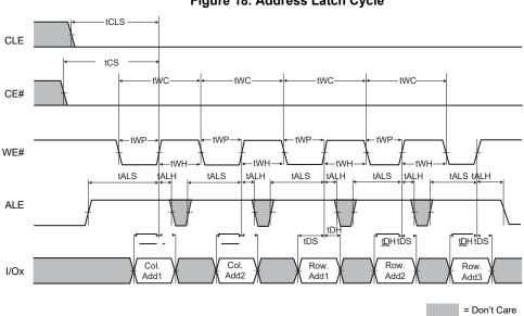
Figure 18. Address Latch Cycle
