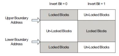
Table 19 illustrates how internally the blocks are being protected for single plane operations (shaded area) when the lower and upper addresses are respectively set to 1 and 4.
