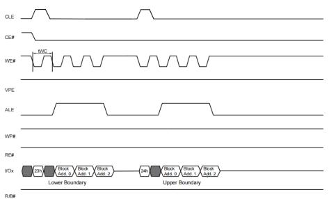
Figure 9. Waveforms for Block Unprotect
