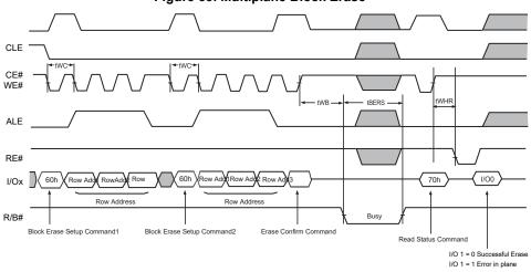
Ex.) Address Restriction for Multiplane Block Erase Operation
