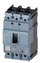
circuit breaker 3VA5 UL frame 125 breaking capacity class S 25kA @ 480 V 3-pole, line protection TM230, FTAM, In=70A overload protection Ir=70A fixed short-circuit protection Ii=5...10 x In UL489 SB (naval), 50 deg. cel. cable connection on both sides
