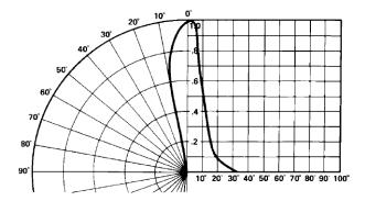
Figure 8: Relative Luminous Intensity vs. Angular Displacement, HLMP-K155
