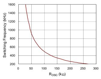
Figure 7. Switching Frequency vs. ROSC Resistor
