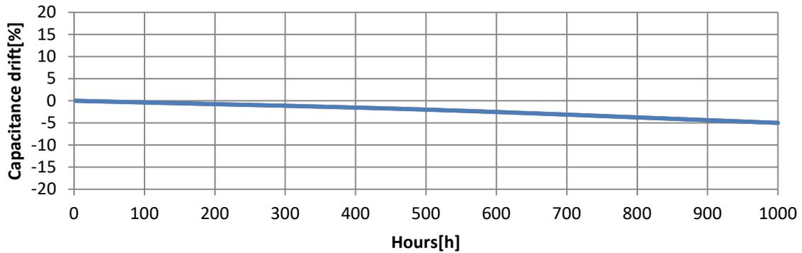
In the testing environment (temperature 85℃ ,relative humidity 85%, 220VAC),During the 500 hours' continuous operating, $c \leq 3\%$ .During the 1000 hours' continous operating, $c \leq 10\%$ . $\text{tg}\delta \leq 3 \cdot 10^{-3}$
