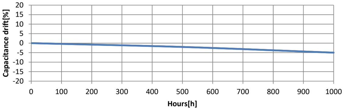
In the testing environment (temperature 85℃ ,relative humidity 85%, 240VAC), During the 500 hours' continuous operating,  $c \leq 3\%$ . During the 1000 hours' continuous operating,  $c \leq 10\%$ .  $tg\delta \leq 3 \times 10^{-3}$
