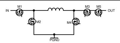
Figure 9-6. Buck-Boost Internal Power FETs
