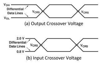
Figure 8-4. USB Endpoint Crossover Voltages
