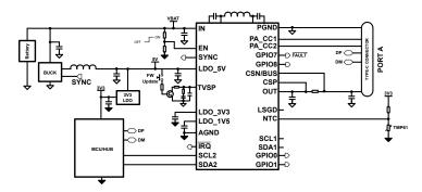
Figure 10-2. Simplified Single USB PD with MCU/HUB
