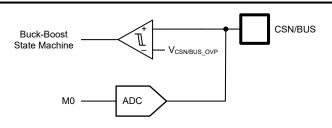
Figure 9-16. V<sub>BUS</sub> OVP and UVP
