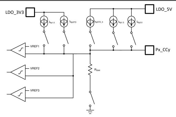
Figure 9-26. Plug and Orientation Detection Block
