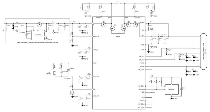
Figure 10-3. TPS25762-Q1 Application Schematic
