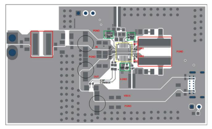
Figure 12-1. TPS25762-Q1 Power Stage Layout
