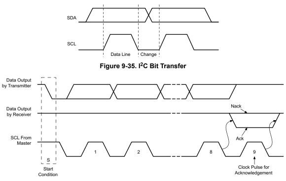
Figure 9-36. I<sup>2</sup>C Acknowledgment
