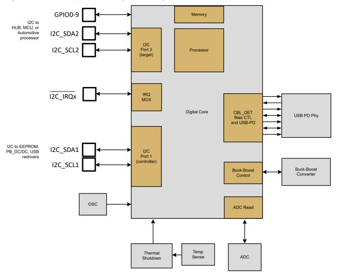
Figure 9-40. Digital Core Simplified Block Diagram
