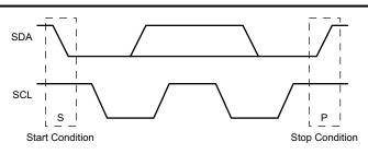
Figure 9-34. I<sup>2</sup>C Definition of Start and Stop Conditions
