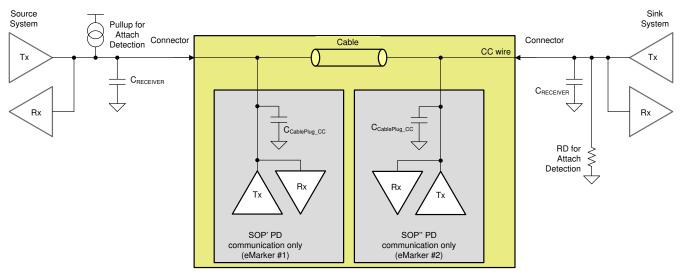
Figure 9-24. Example USB-PD Multi-Drop Configuration
