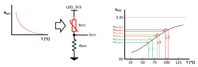
Figure 9-42. NTC Response Curve
