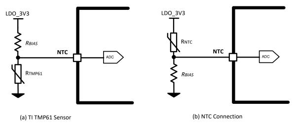
Figure 9-41. Thermistor Connections (a) PTC, (b) NTC
