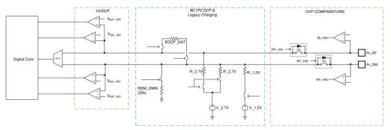
Figure 9-31. BC1P2 Functional Diagram
