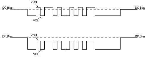
Figure 9-22. TX Driver Transmission with DC Bias
