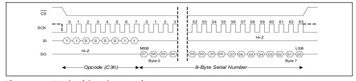
Figure 18 Read serial number operation
