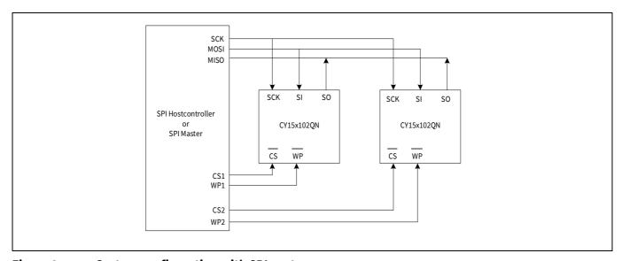
System configuration with SPI port Figure 2
