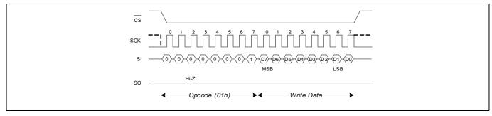
Figure 9 WRSR bus configuration (WREN not shown)
