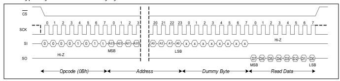
Figure 12 Fast read operation
