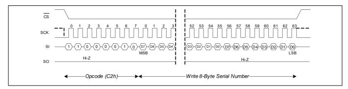
Figure 17 Write serial number (WREN not shown) operation
