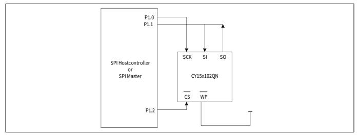
System configuration without SPI port Figure 3
