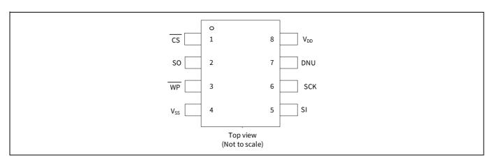
Figure 1 8-pin SOIC pinout
