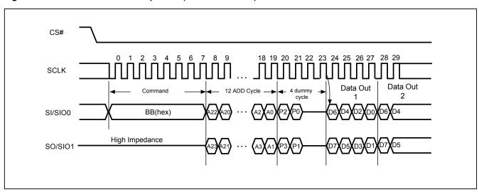
Figure 19. 2 x I/O Read Mode Sequence (Command BBh)
