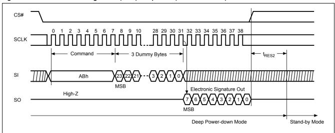
Figure 30. Read Electronic Signature (RES) Sequence (Command ABh)
