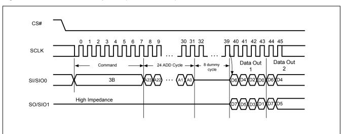
Figure 18. Dual Read Mode Sequence (Command 3Bh)
