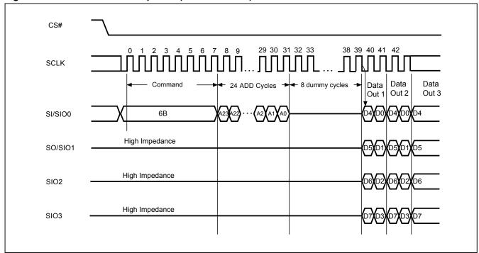
Figure 20. Quad Read Mode Sequence (Command 6Bh)
