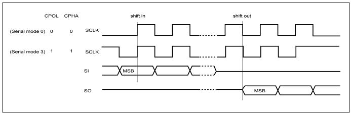
Figure 1. Serial Modes Supported
