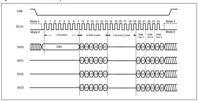
Figure 21. 4 x I/O Read Mode Sequence
