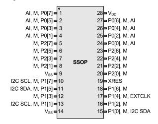
**LEGEND** A = Analog, I = Input, O = Output, and M = Analog Mux Input.
