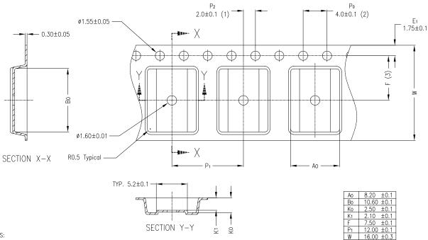
Figure 12. 28-Pin SSOP Carrier Tape Drawing
