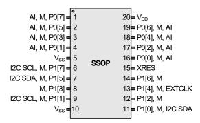
**LEGEND** A = Analog, I = Input, O = Output, and M = Analog Mux Input.
