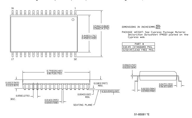
Figure 10. 32-pin TSOP II (20.95 × 11.76 × 1.0 mm) ZS32 Package Outline, 51-85095
