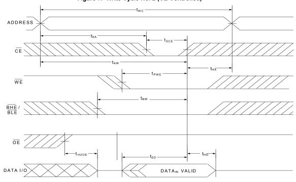
Figure 8. Write Cycle No. 3 (WE Controlled, OE LOW) [27, 28, 29]
