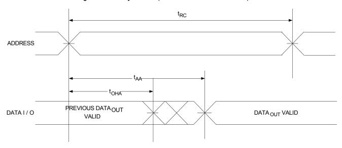
Figure 5. Read Cycle No. 2 (OE Controlled) [22, 23]
