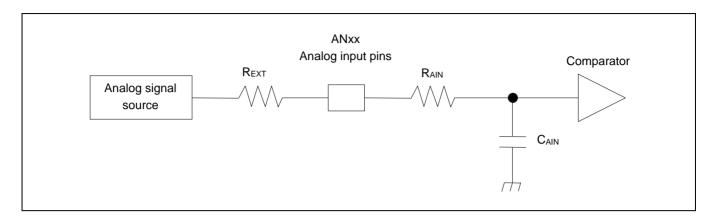
(Equation 1)  $t_S \ge (R_{AIN} + R_{EXT}) \times C_{AIN} \times 9$
