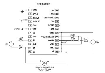
Figure 20: Propagation Delay Test Circuit
