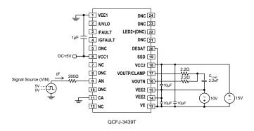
Figure 22: CMR Output Low Test Circuit
