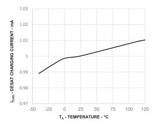
Figure 19: I<sub>DSCHG</sub> vs. Temperature
