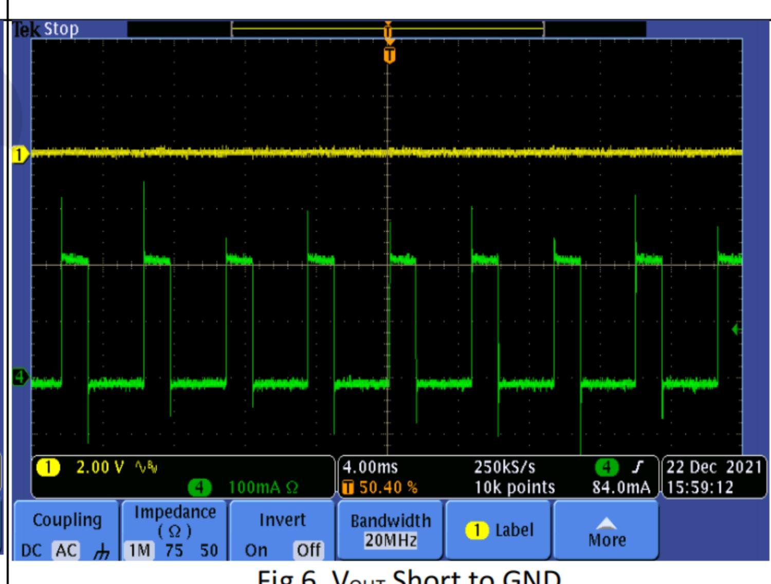
Fig 6. V<sub>OUT</sub> Short to GND
