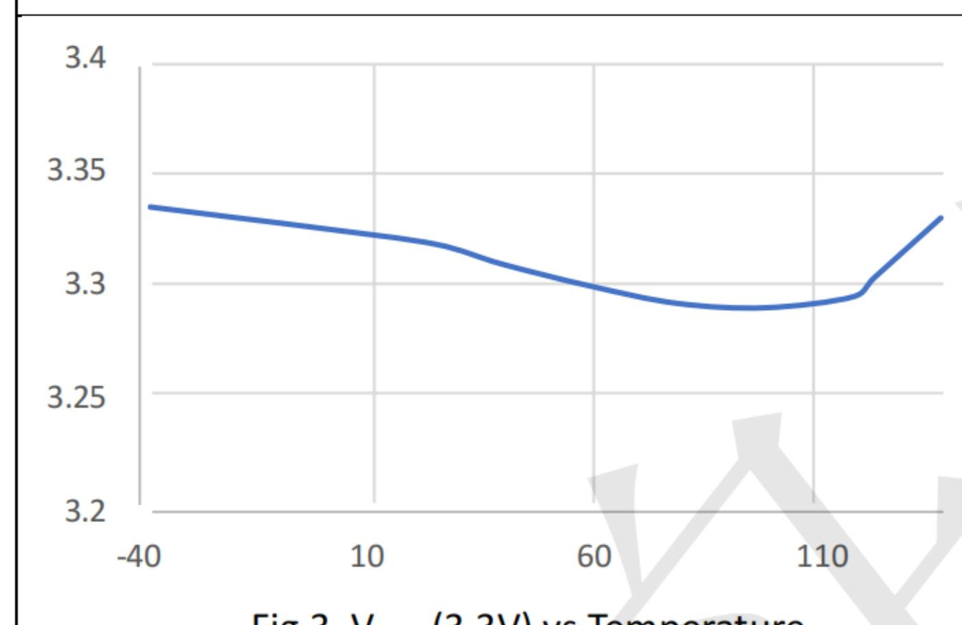
Fig 3. V<sub>OUT</sub> (3.3V) vs Temperature
