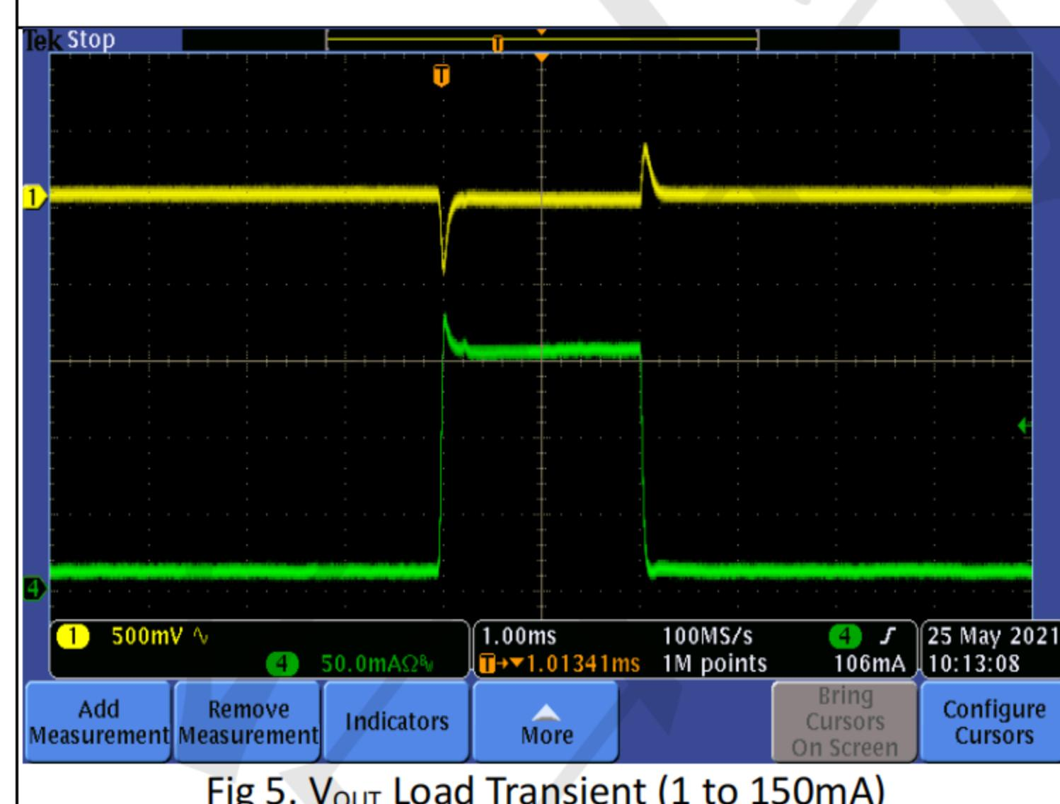
Fig 5. V<sub>OUT</sub> Load Transient (1 to 150mA)
