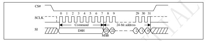
Figure 10-31a Block Erase (BE) Sequence (QPI)
