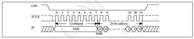
Figure 10-36aBuffer Load Sequence (QPI)
