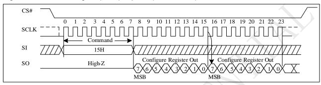
Figure 10-6a Read Status Register (RDCR) Sequence (QPI)
