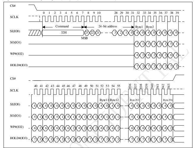
Figure 10-34 Quad Page Program (QPP) Sequence (Command 32h)
