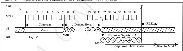
Figure 10-44 Read Electronic Signature (RES) Sequence (Command ABh)
