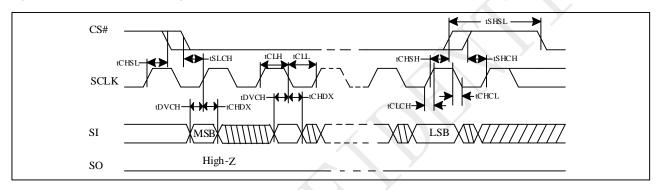
Figure 5-5 Output Timing
