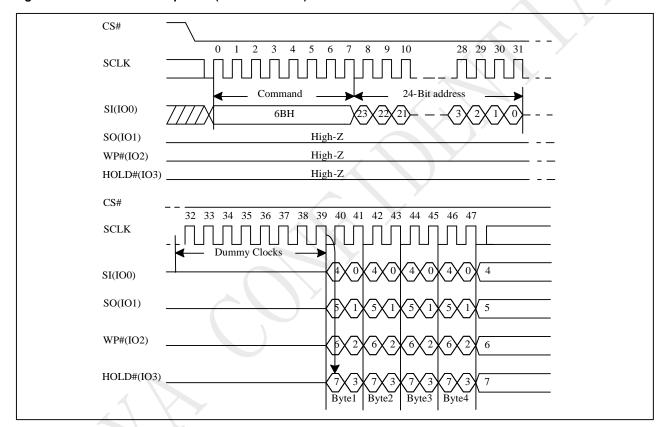
Figure 10-17 Quad Read Sequence (Command 6Bh)
