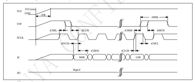
Figure 5-9 Power-up Timing
