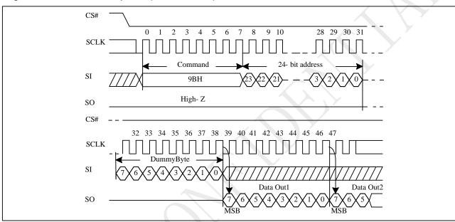
Figure 10-37Buffer Read Sequence (Command 9Bh)
