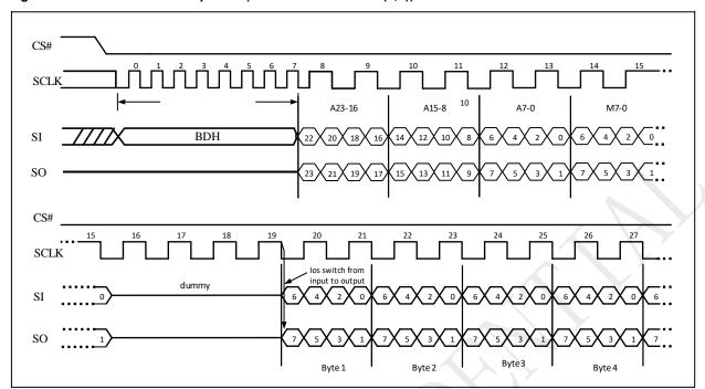
Figure 10-16DTR 2IO Read Sequence (Command BDM5-4 ≠ (1,0))
