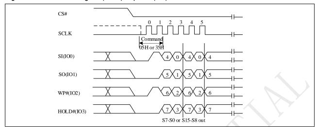
Figure 10-5a Read Status Register (RDSR) Sequence (QPI)
