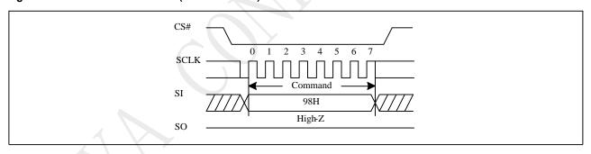
Figure 10-57a Global Block Unlock (QPI)
