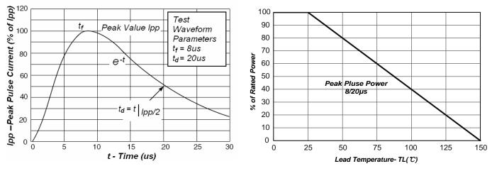
Fig1. Pulse Waveform
