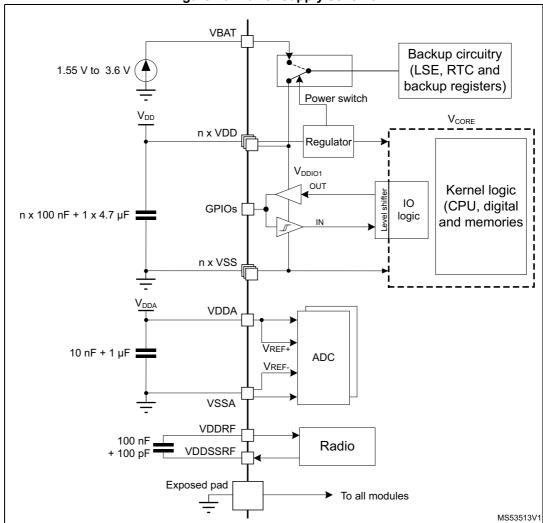
Figure 10. Power supply scheme
