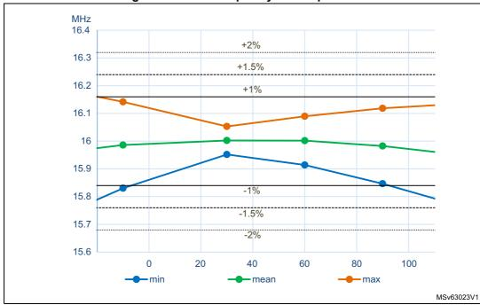
Figure 16. HSI16 frequency vs. temperature
