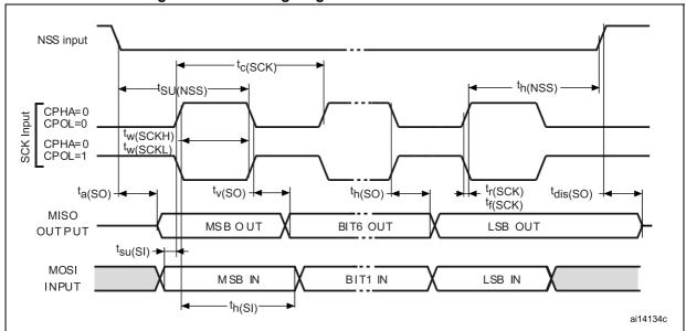
Figure 23. SPI timing diagram - slave mode and CPHA = 0
