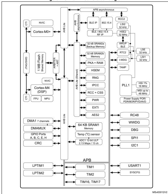
Figure 1. STM32WB50CG block diagram
