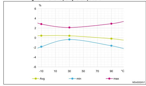
Figure 18. HSI48 frequency vs. temperature
