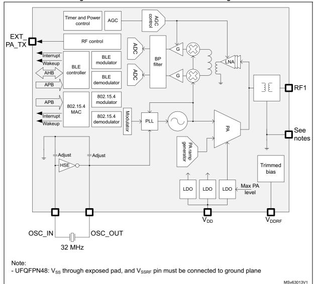
Figure 2. STM32WB50CG RF front-end block diagram
