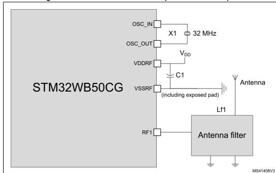
Figure 3. STM32WB50CG external components for the RF part
