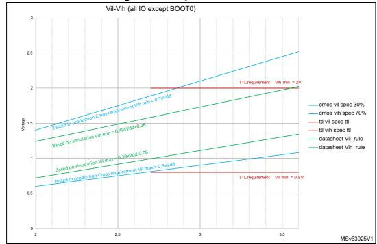
Figure 19. I/O input characteristics
