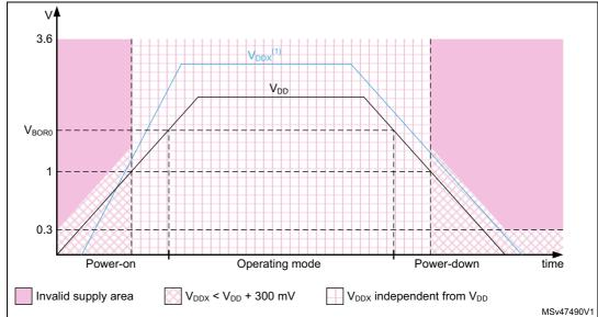
Figure 4. Power-up/down sequence
