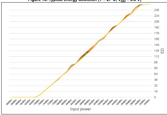
Figure 13. Typical energy detection (T = 27°C, V<sub>DD</sub> = 3.3 V)
