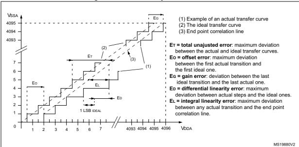
Figure 21. ADC accuracy characteristics
