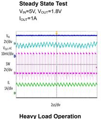
1A LOAD  $V_{\rm IN}$ 2V/div  $V_{\text{OUT}}$ .ac 10mV/div SW 2V/div IL 1A/div 2us/div
