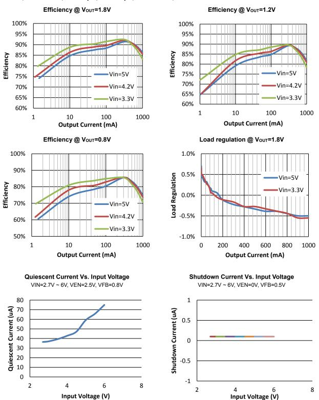
$V_{IN}$  =5V,  $V_{OUT}$  = 1.8V, L = 1.5µH, C2 = 22µF, TA = +25°C, unless otherwise noted
